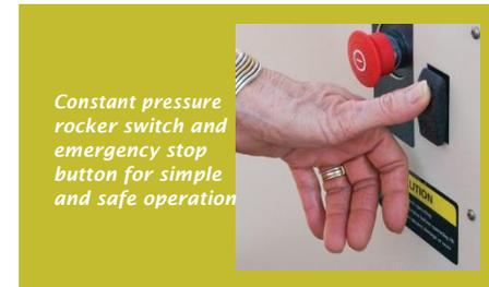
Constant pressure rocker switch and emergency stop button for simple and safe operation
